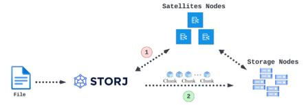
Fig. 3: The overlay network architecture used by Storj.
