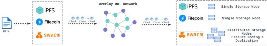
Fig. 2: The overlay network architecture used by Filecoin, IPFS, and Swarm.
