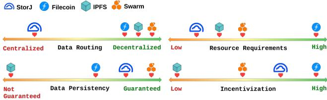
**Fig. 1:** Design choices of IPFS, Storj, Swam, and Filecoin that falls on spectrum of centralized-to-decentralized data routing strategies, guaranteed-to-not guaranteed data persistency, high-to-low resource requirements, and high-to-low incentivization.
