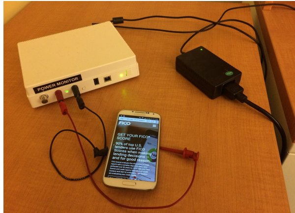
Fig. 3. Our hardware setup showing the Samsung S4 under test connected to the Monsoon power monitor.
