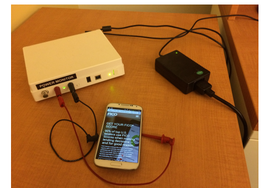
Using a power monitor to get P_s just for building the model
